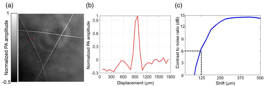
**Fig. 2** In-plane resolution quantification. (a) PA image of three crosswise tungsten wires. (b) The photoacoustic amplitude distribution along the red line in (a). (c) The CNR versus the shift in the sum of the original line profile shown in (b) and the shifted one. The in-plane resolution, defined as the shift corresponding to 6-dB CNR, is 125  $\mu\text{m}$ .
